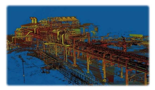
he majority of CAD softwares will allow these files to be read, provided that an appropriate module is added. For example, PDMS, PDS, SmartPlan, Autocad, Microstation, 3DSMax, etc. can import millions of points, with no difficulty, using a plug-in such as Pointools or Lasergen.
